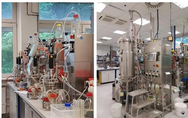
**Figure 3:** Our fermentation lab allows piloting up to a scale of 150L
